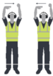
APU Connected APU Disconnected
